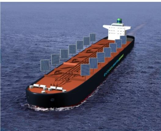
the wind and sun. The array of rigid sails (which are based on EMP's EnergySail™ technology) will be automatically positioned by a computer system to best suit the prevailing weather conditions and can be lowered and stored when not in use or in bad weather.
