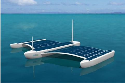
The Aquarius USV is being developed as a cost-effective unmanned surface vessel (USV) that will incorporate a number of technologies from Eco Marine Power & its strategic partners. These technologies include the EnergySail, marine computer systems & lightweight flexible marine solar panels.
