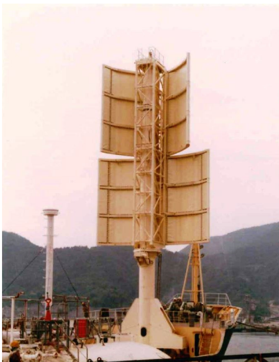
Figure 5: Folding JAMDA sail manufactured by Teramoto Iron Works on a ship in the 1980's
